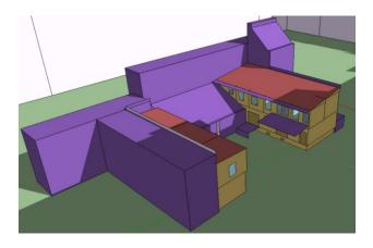
Figure 1: EnergyPlus model of the courtyard building
