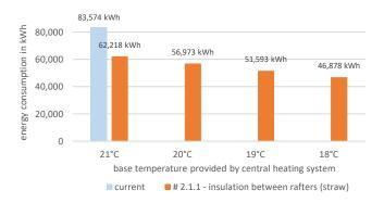
Figure 7: Energy demand for different base temperatures
